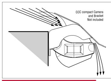
Install the cover in such a way that the air stream in front of the camera creates an overpressure; to prevent dirt on the lens.
